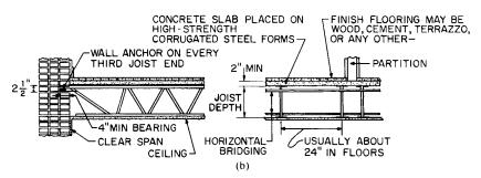
FIGURE 8.23 Some examples of open-web steel-joist floor construction.
