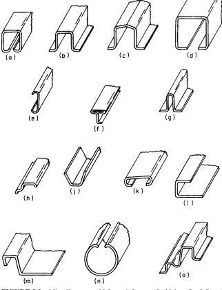
**FIGURE 8.2** Miscellaneous cold-formed shapes. (Bethlehem Steel Corp.)
