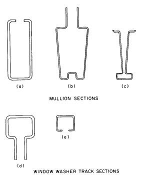
FIGURE 8.3 Cold-formed stainless steel sections. (The International Nickel Co., Inc.)
