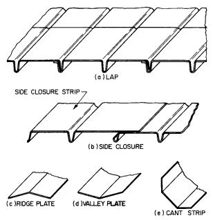
FIGURE 8.16 Roof-deck details.
