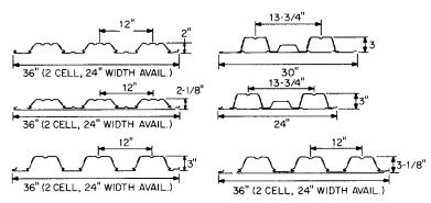
**FIGURE 8.17** Composite cellular and fluted steel floor sections. (*Courtesy H. H. Robertson Co., Ambridge, Pa.*)
