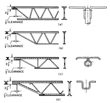
FIGURE 8.22 Some examples of open-web steel joists.
