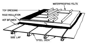
FIGURE 8.13 Roof-deck assembly.
