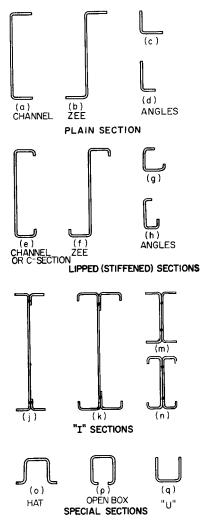
**FIGURE 8.1** Typical cold-formed steel structural sections
