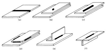
**FIGURE 8.10** Types of sheet-steel welds: (a) square-groove weld: (b) arc spot weld (round puddle weld); (c) arc seam weld (oblong puddle weld); (d) fillet welds; (e) flare bevel-groove weld; (f) flare V-groove weld.
