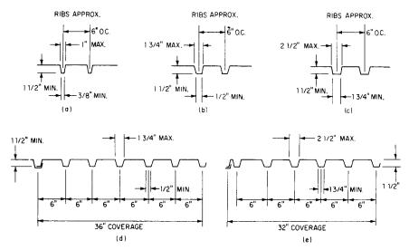
**FIGURE 8.14** Typical cold-formed steel roof-deck sections. (a) Narrow rib: (b) intermediate rib; (c) wide rib; (d) intermediate rib in 36-in-wide sheets with nested side laps; (e) wide rib in 32-in-wide sheets with upstanding seams.
