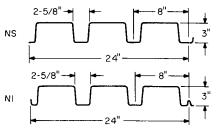
**FIGURE 8.15** Cross sections of types NS and NI roof deck for 9- to 15-ft spans.
