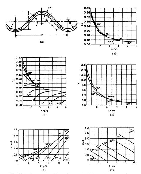
**FIGURE 8.19** Factors for determining section properties of the arc-and-tangent type of corrugated steel sheet shown in (a).
