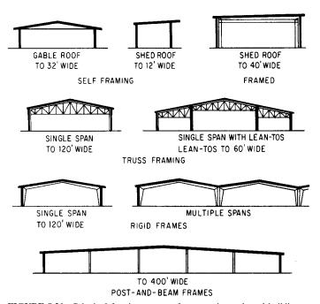
FIGURE 8.21 Principal framing systems for preengineered steel buildings.
