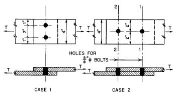
FIGURE 8.11 Bolted connections with two bolts.
