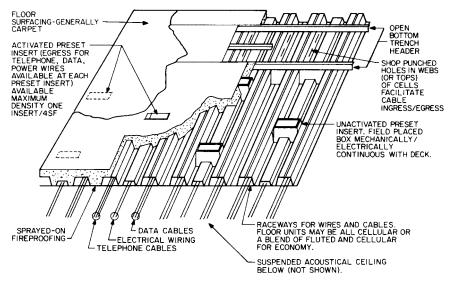
**FIGURE 8.18** Composite cellular and fluted steel floor sections. (*Courtesy H. H. Robertson Co., Ambridge, Pa.*)
